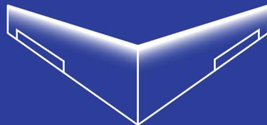
**5. Swing-wings** are wings that swing backward from a straight wing at low speed to a sweepback wing at high speed. They take advantage of the benefits of both types of wings.
