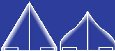
**3. Sweepback wings** are used for most high-speed aircraft. They create less drag but are less stable at low speeds. The wings on commercial jets have a lower sweep than those on high-speed fighters.
