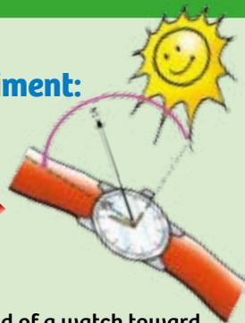
Point the hour hand of a watch toward the sun. Hold it in place and imagine a line that is exactly between the 12 o'clock mark and the hour hand. This line points out of the watch center, toward the south.
