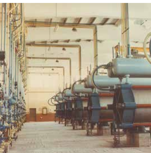
Production of hydrogen according to the pressure electrolysis method (Photo: Lurgi, Frankfurt am Main)
