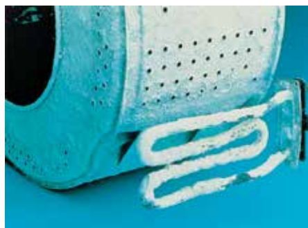
In a short time, the heat in the washing machine leads to the precipitation of limestone (calcium carbonate) on the heating element (photo: Benckiser Deutschland GmbH, Mannheim).
