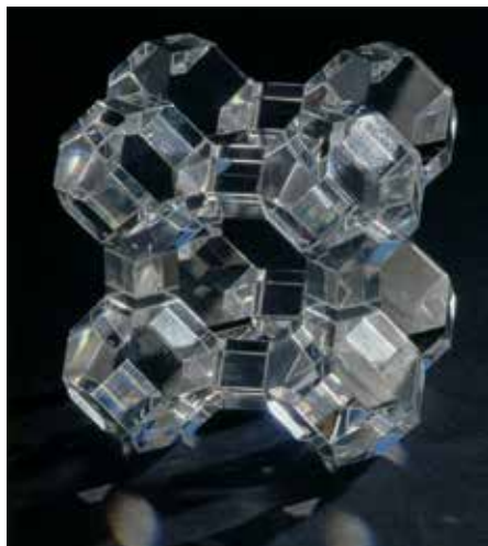
This "cage molecule" (zeolite A) contains sodium ions that are exchanged for the troublesome calcium ions contained in hard water. Sodium ions are not disruptive during the washing process (photo: Henkel KgaA, Duesseldorf).
