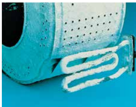
Calcium deposits on the heating elements of a washing machine (photo: Benckiser)
