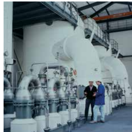
Evaporator in which the brine is heated until the table salt crystallizes out (photo: Saline Bad Reichenhall, Germany).
