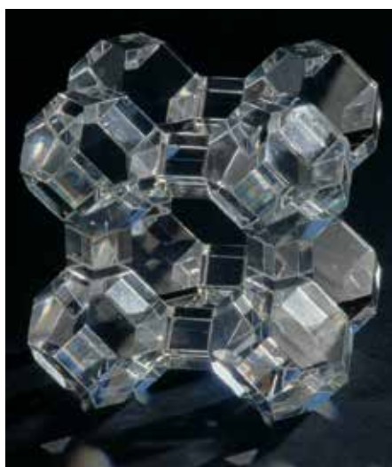
"Cage molecule" of zeolith A. The molecule consists of an aluminum-silicon framework that contains sodium ions. Its effect as a softener derives from an exchange of calcium ions for sodium ions (photo: Henkel).
