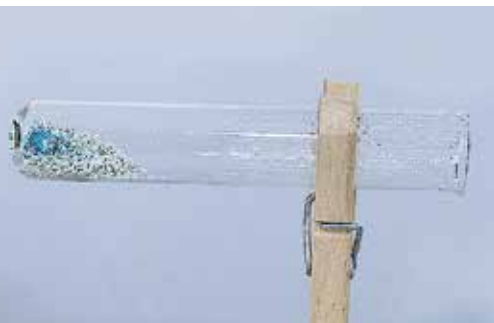
When the blue copper sulfate crystals are heated, you get white copper sulfate free of water of crystallization.
