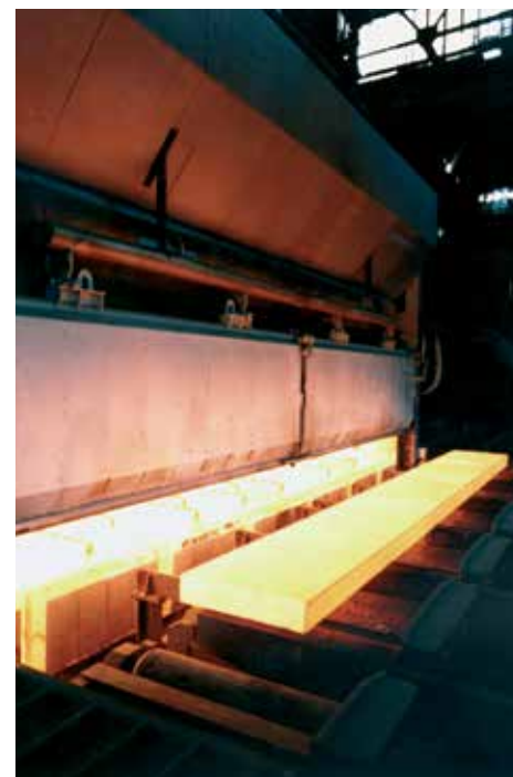
Images from steel production Left: Tapping raw iron from the furnace. Middle: In the converter, the carbon component of the iron is reduced to 1.7% by blowing in oxygen. Impurities (such as sulfur and phosphorus) are bound to additives and separated out as slag. Right: On the rolling mill, glowing blocks of steel are processed into steel girders, sheet metal, and other products. (Photos: ThyssenKrupp Steel)
