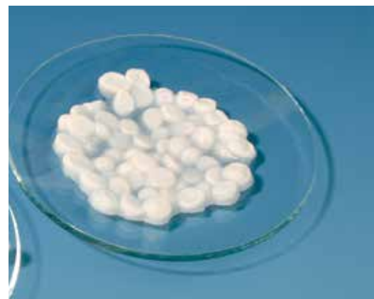
Sodium hydroxide draws humidity from the air and dissolves.
