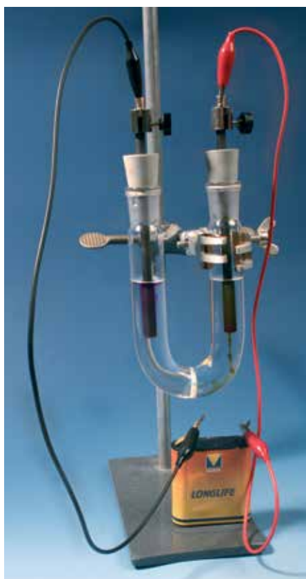
Electrolysis of a potassium iodide solution
