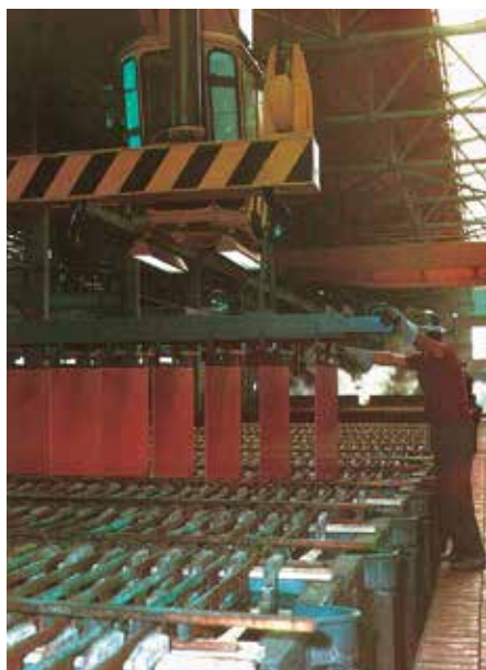
Industrial copper refining through electrolysis; the copper separates out onto the suspended plates (photo: Lurgi).
