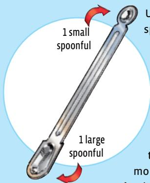
Use the double-headed measuring spoon, which has a large end and a small end, to take chemicals from the vials. A “large” spoonful means one level scoop from the larger end, while a “small” spoonful means a level scoop from the small end. Sometimes a “spoon tip” will be enough, meaning no more than half of the small end, or preferably even less. Always make sure you close the vial immediately after each use!
