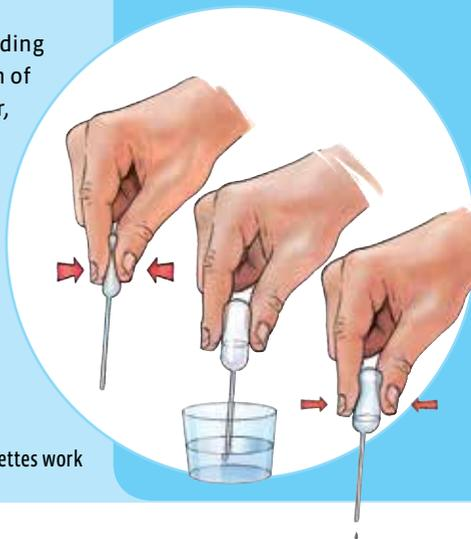
How the dropper pipettes work
