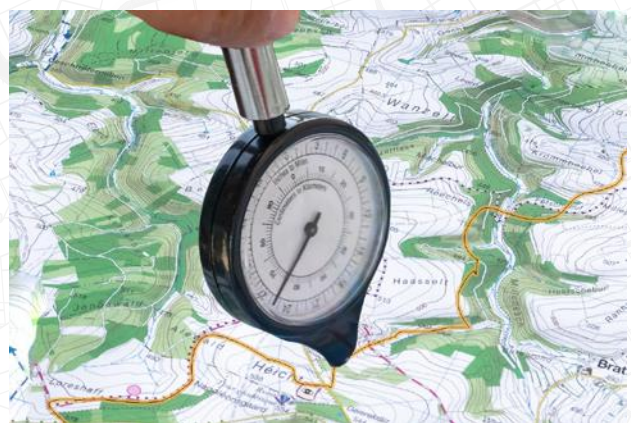
Pic 4. Measuring lines with a curvimeter
